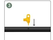
Use the Key Punch to punch hole in 13mm Poly Pipe for emitter installation.
