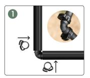
Slide 13mm Ratchet Clamp over Poly Pipe. Then, push barbed fittings into tubing, slide ratchet clamps over joins to secure.
