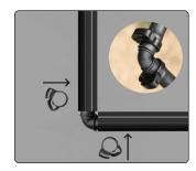
4 Once all Elbow, Tee and Joiners are connected, use the Hold-Down Stakes to secure the 13mm Poly Pipe to the ground.
