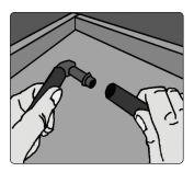
3 Place 13mm Ratchet Clamps over the Poly Pipe before attaching the barbed fittings. Push barbed fittings into the 13mm Poly Pipe, securing each end of the fittings with a 13mm Ratchet Clamp. Repeat until all fittings are attached.
