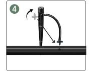
Snap off adaptor, insert into 4mm tube, push micro feeder tube into Adjustable Drip Spike and adaptor into 13mm Poly Pipe.
