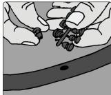
2 Snap off the included adaptor from the Adjustable Drip Spike.
